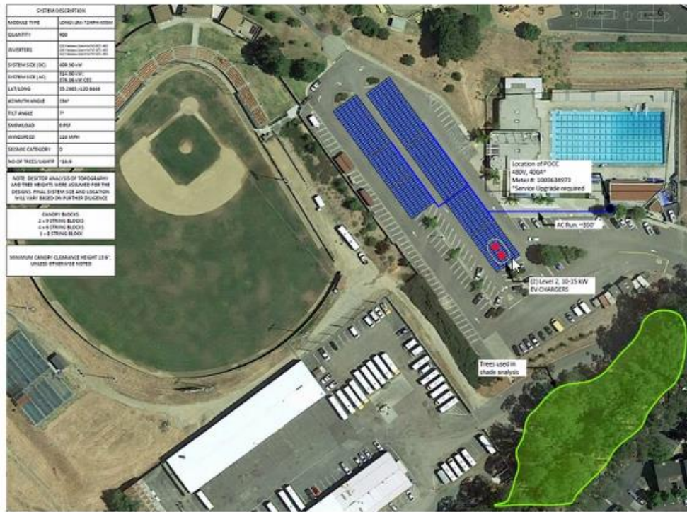
Figure 20: SLO Swim Center Solar PV Layout
