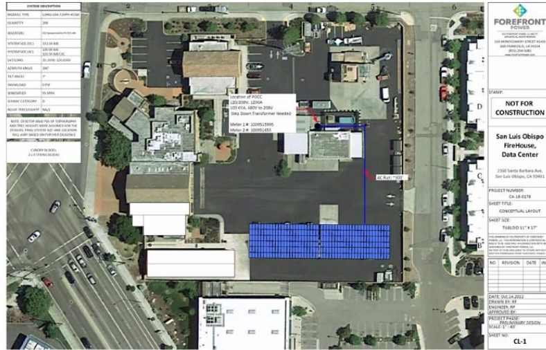
Figure 22: Fire Station 1 Solar PV Layout
