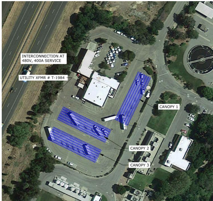
Figure 21: Bus Yard Solar PV Layout
