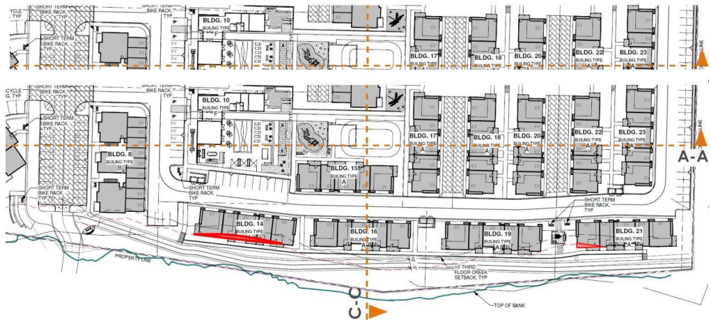
Figure 5: Portions of Building 14 and 21 encroachment within the 35-foot creek setback.
