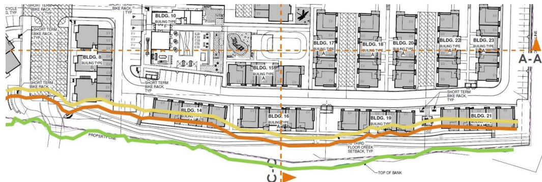
Figure 3: Top of Bank (green), 35-foot creek setback (orange), and an additional 10-foot upper story step back (yellow).
