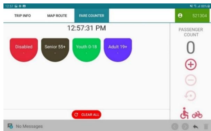
Image - Fare Counting – Manual input of passengers by the driver. Great for sampling and testing APC accuracy.
