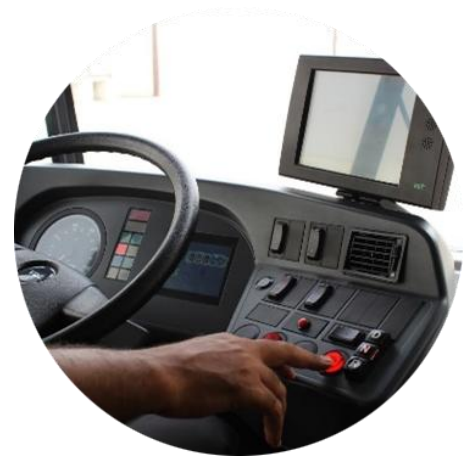
Image - Our proposed Covert Alarm. The hardware can be placed in the City’s preferred location.
