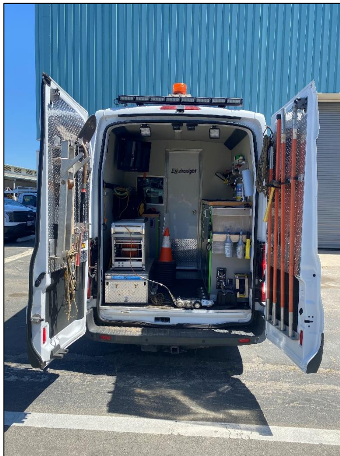
Figure 1: Existing CCTV Van With Camera Equipment
