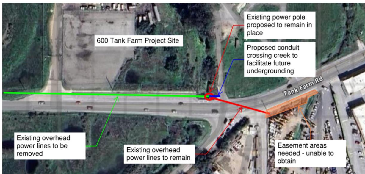
Figure 2: Proposed Utility Undergrounding Revisions Design Concept: Tank Farm Road
