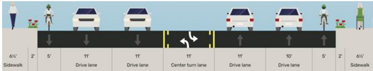
Existing Cross Section of Tank Farm Rd: Broad St to Poinsettia St
