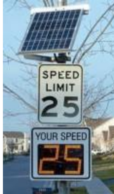
Example of Radar Speed Feedback Sign
