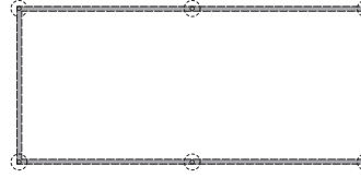
5 UNIT B: HELICAL PIER FOUNDATION PLAN Scale: 1/4" = 1'-0" FOR MORE INFORMATION, REFER TO SHEET JRSC-C FOR HELICAL PIERS: CONCEPTUAL PLAN
