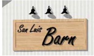
B1 MARKET BUILDING SIGNAGE WOOD AND STEEL DIMENSIONS: 5'-6"H x 14"W 77 SF (QTY 2) COLOR: BLACK OR WHITE
