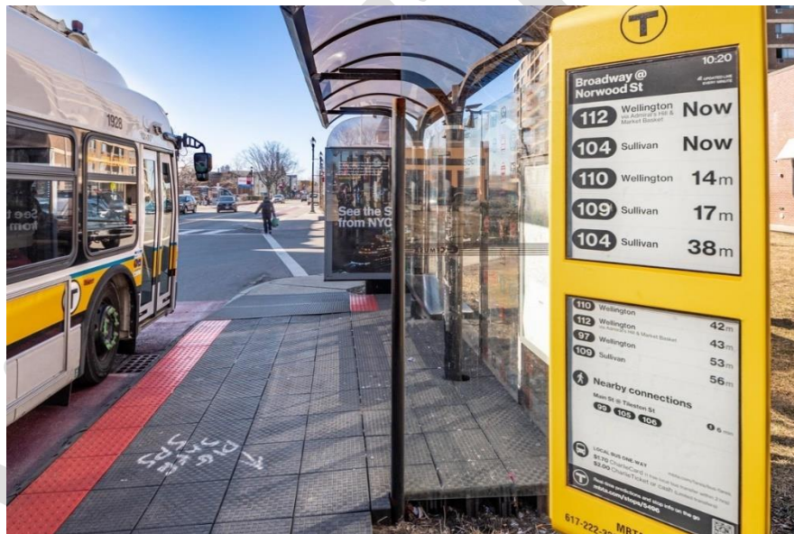
Figure 3. An example of an RTPI sign at a Massachusetts Bay Transportation Authority (MBTA) Implementation Bus Stop
