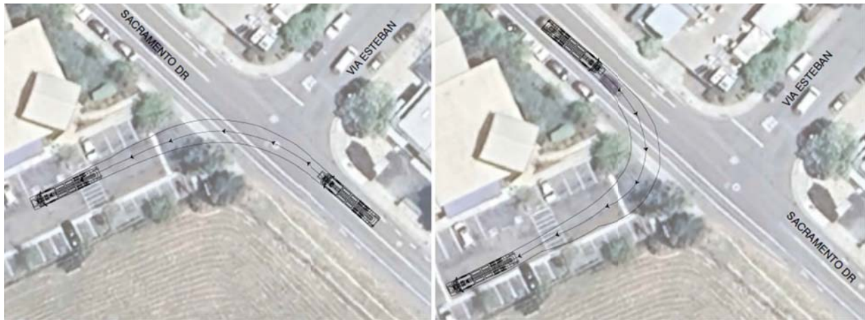
Figure 11: Emergency Vehicle Access onto Project Site
