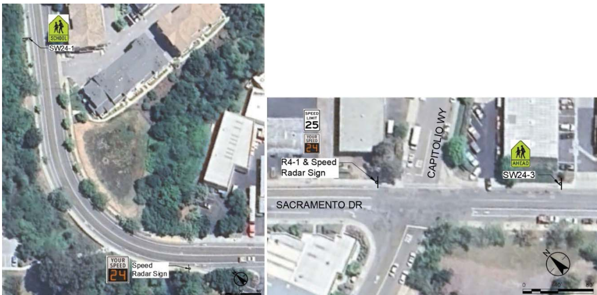
Figure 5: Proposed Treatments north (left) and south (right) of the project site
