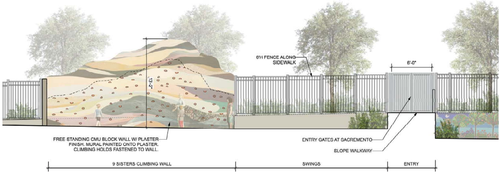
1 LOOKING EAST TOWARD CLIMBING WALL Scale: 1/4" = 1'-0"
