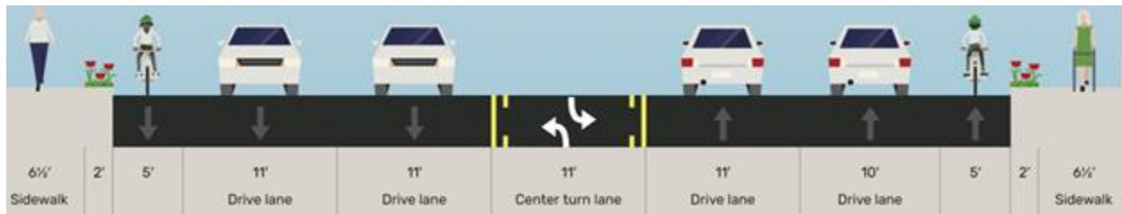
Existing Cross Section of Tank Farm Rd: Poinsettia St to Righetti Ranch Rd
