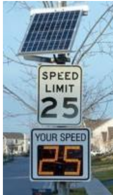
Example of Radar Speed Feedback Sign
